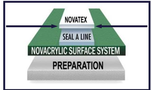
**NOTE: Seal-A-Line before application of Novatex is recommended**
