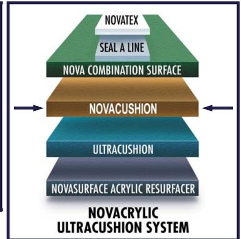
After the application of NOVACUSHION is completed, 2 coats of COMBINATION SURFACE should be applied. This results in a uniform texture and appearance.
