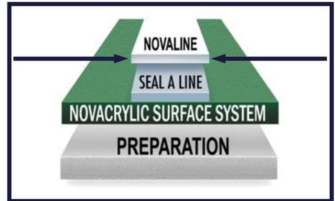
**NOTE: Seal-A-Line before application of Novaline is recommended**
